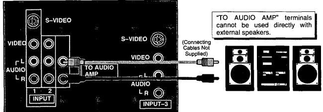
Adjustment – When an audio amp is connected to "TO AUDIO AMP" terminals:
